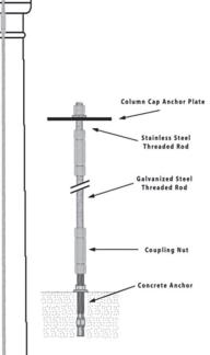
**IMPORTANT WARRANTY NOTE:** DO NOT ANCHOR THIS PRODUCT TO PAVERS OR TILE OF ANY TYPE. ANCHOR HARDWARE SHOULD ANCHOR COLUMNS TO SOLID CONCRETE PAD, CONCRETE FOOTER OR WOOD/COMPOSITE DECKING. COLUMN SHAFTS MUST REST ON FLAT SOLID CONCRETE OR DECKING AND PAVERS CAN BUTT-UP AGAINST SHAFT AND DECORATIVE BASE CAN HIDE SEAMS.
