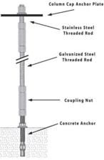
**IMPORTANT WARRANTY NOTE:** DO NOT ANCHOR THIS PRODUCT TO PAVERS OR TILE OF ANY TYPE. ANCHOR HARDWARE SHOULD ANCHOR COLUMNS TO SOLID CONCRETE PAD, CONCRETE FOOTER OR WOOD/COMPOSITE DECKING. COLUMN SHAFTS MUST REST ON FLAT SOLID CONCRETE OR DECKING AND PAVERS CAN BUTT-UP AGAINST SHAFT AND DECORATIVE BASE CAN HIDE SEAMS.
